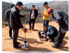
Determine the bearing capacity and compaction quality of soils and non-cohesive subbases fast, reliably and precisely.
