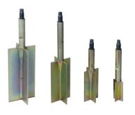
The registration of the maximum torque T<sub>max</sub> is possible due to the use of a precise torque wrench. The technique of testing with the conical vane SLVT is therefore a combination of probing with a dynamic probe DPL with the possibility of measuring the shear strength c<sub>fv</sub> at the same time.
